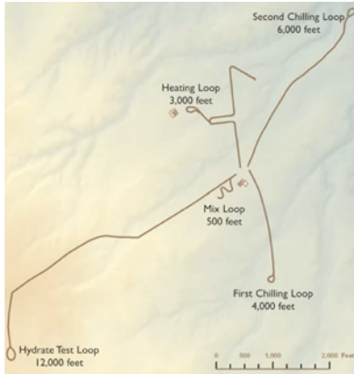
Basic schematic of the deepwater test loop to be used in the upcoming AOT™ testing.
