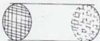
Fig.4 Two copper meshes are inserted inside the fuel line.
